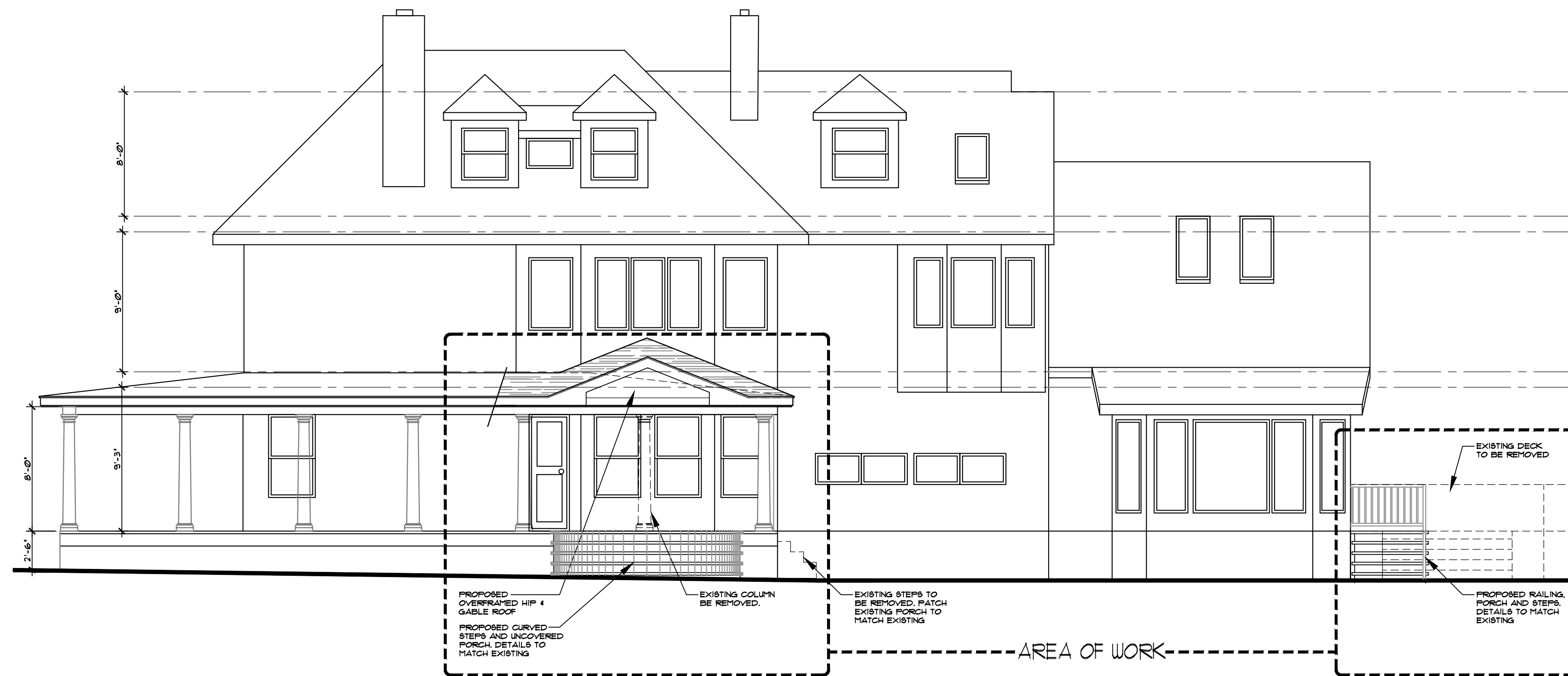
2 PROPOSED EXTERIOR ELEVATION- POOL SIDE SCALE: 1/4" = 1'-0"
